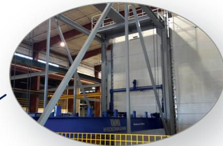
Full automatic **storage and retrieval** crane and curing chamber. Heating by computer controlled hot air ventilation.
