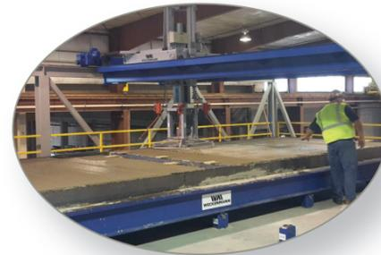
**Power troweling** on top of the curing chamber. Provides best surface qualities on top.
