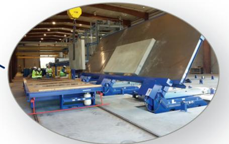
**Tilting station** to bring the pallet to an almost vertical position for shipping wall panels.
