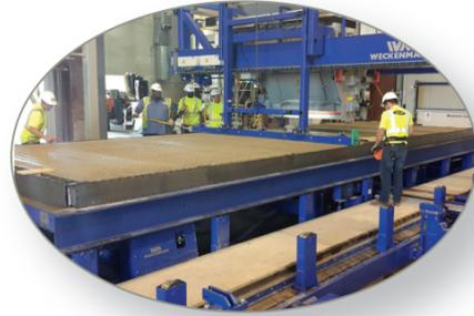
**Concrete compaction** by low frequency oscillation.
