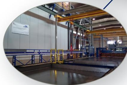
Stations for set up **side rails** with integrated magnets (Type M-Basic / M-Top). Standard depths 6", 8", 10", 12"
